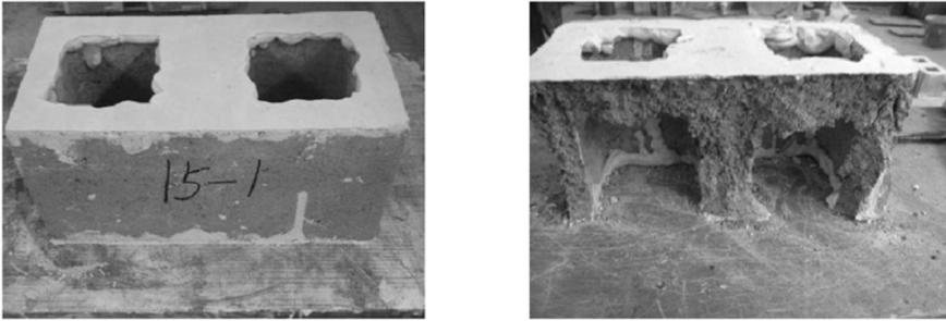
Fig. 3. Setting and destruction of building blocks
