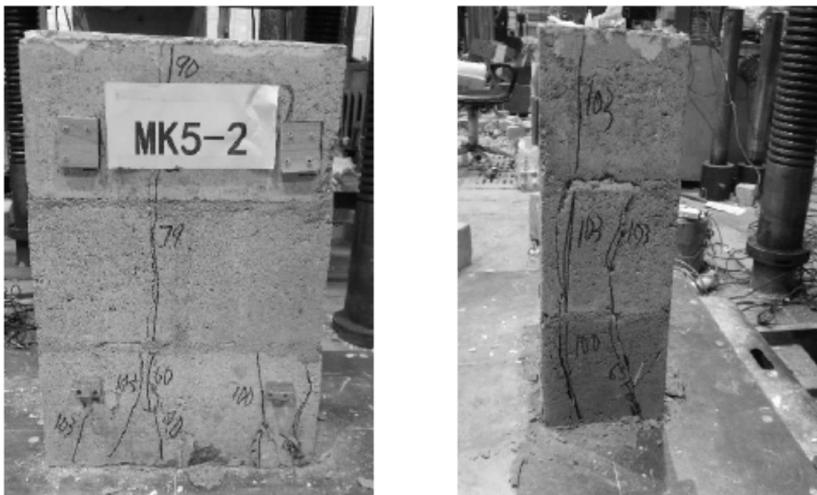
Fig. 4. Failure state of hollow compression standard parts
